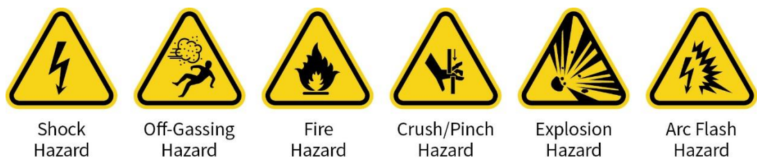
Figure 11-1: Common Hazard Labels Associated with BESS
