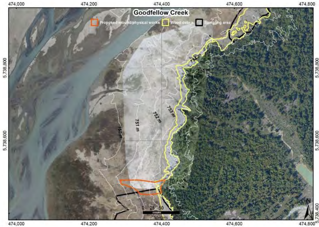
Figure 5-12: Schematic of proposed mound location (orange polygon) at Goodfellow Creek. The distribution of wood debris relative to the mound construction site is shown. The location and shape of the mound is approximate.
